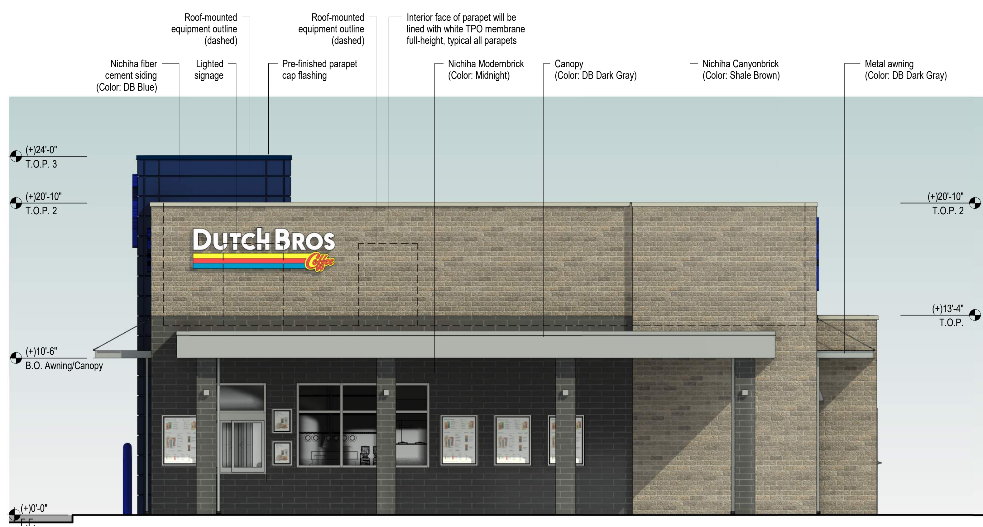
North Elevation - (Walk-Up Elevation) 1/4" = 1'-0"
